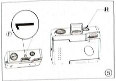
Continue to advance the film by turning the film advance wheel until it stops. Press the shutter button (H). Repeat this procedure one more time. The Film Counter (F) will now show number "1", and the camera is ready for taking pictures.
