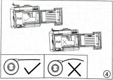
Ensure that the film lays flat against the center of the camera and close the camera's back door.
