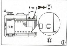
Pull out the film from the film canister, insert the film leading edge into take-up spool.and hook the hole onto the film take-up spool  $\bigcirc$ . Slightly advance the film by turning the film advance wheel  $\bigcirc$ .
