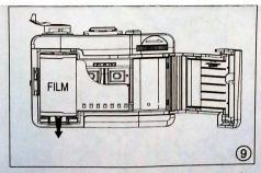
Open the camera back door and remove the film for processing.
